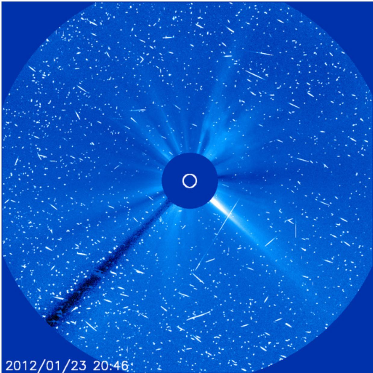
Figure 3 – This figure shows the effects of high-energy solar protons on an exposed imager on the Solar and Heliospheric Observatory during the January 23, 2012 solar storm. A greatly reduced flux of particles entering shielded satellite circuitry results in SEUs, many of which are harmless, but a few per year can result in serious operational anomalies.
