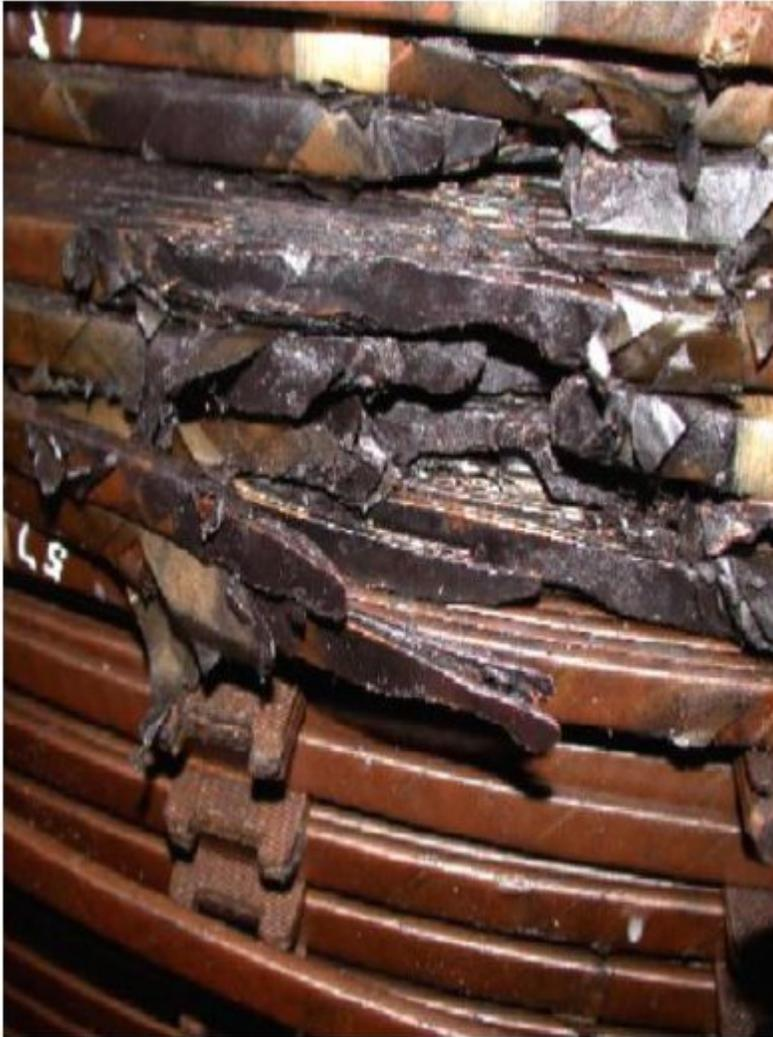
Figure 6- GICs cause damage to large transformers through magnetostriction and the resulting thermal heating. This picture is reminiscent of the images of transformers that failed during the 1989 Quebec Blackout (Courtesy Murtagh, 2009)
